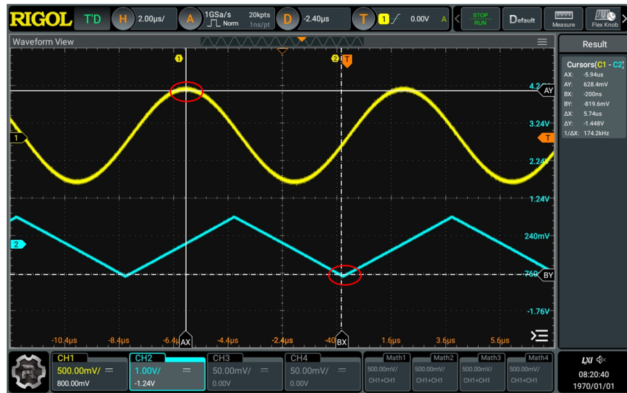
Figure 10.13 Track Measurement (after Horizontal Expansion)
