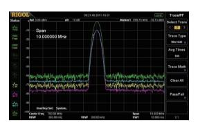
Measure lower level signal with the preamplifier turn on
