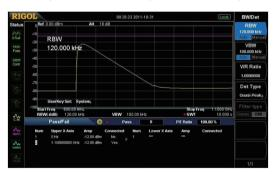
Zero span to demodulate the AM signal
